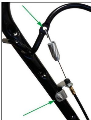
7. The throttle cable MUST be adjusted after installation.
