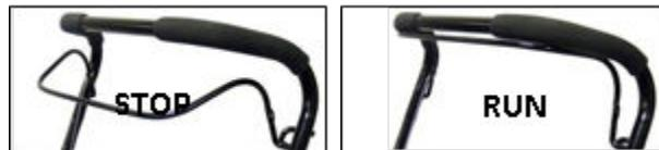
**2. Engine On/Off Switch / Throttle Cable**
